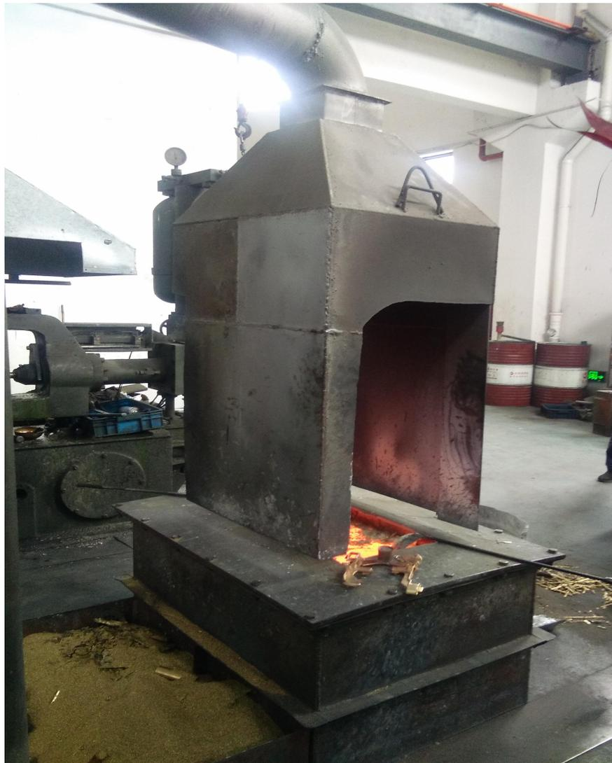
熔化炉及集气罩
